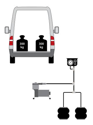
All included: Each of our additional air suspension systems include a high-performance compressor and an in-cab control unit with single or double pressure gauge in the scope of delivery. This enables you to easily and conveniently monitor the air pressure in your air suspension system from the cab and adjust it as necessary.
