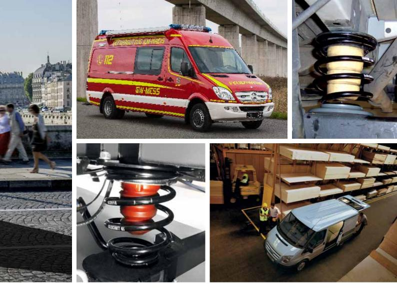
In addition to our leaf springs (page 8), coil springs can be used as additional spring reinforcement in transporter vans and motorhomes operated with a high rear axle load. The coil springs are used in addition to the leaf springs on the rear axle. This raises the overloaded vehicle rear end, considerably enhances ride comfort and minimises side wind sensitivity which specifically has unpleasant effects on the handling of vehicles with a high centre of gravity.
