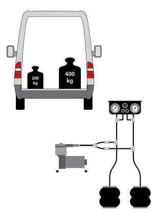
Always keep an eye on things: To ensure you have a complete overview of your system at night, we also offer our illuminated pressure gauges as an optional upgrade package. The integrated LED illumination lets you keep an eye on your air suspension system, even at night. An integrated pressure switch also provides a visual warning of a drop in pressure in the air suspension system.
