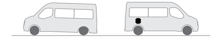
On vehicles with a high rear axle load, the standard steel springs are often overwhelmed. The rear of the vehicle drops down, negatively affecting the suspension comfort. The auxiliary air springs raise the rear end and ensure sufficient spring travel. For unsettled loads, the air bags offer flexibility for filling and emptying.
