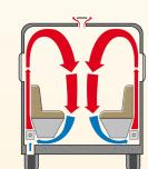
The convectors that are located by the outer walls heat the air. It then rises and heats up walls and furnishings.
