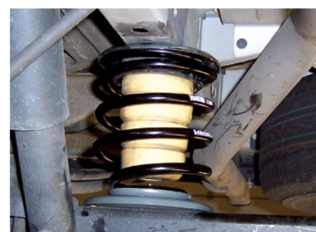
Auxiliary coil springs for the rear axle are used in addition to the standard suspension, as the name suggests.
