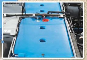
The large water tanks are mounted in the heated double floor insulated with a double-sided aluminium sandwich and so won't freeze at sub-zero temperatures. The water tanks can be removed and replaced via the rear garage.
