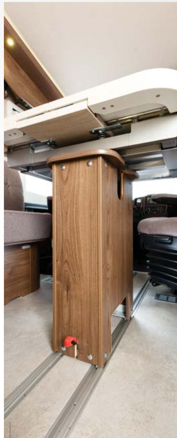
Variable size and position: the unique, sliding table base with pull-out, extendible table top.
