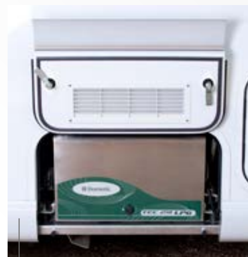
Dometic Tec 29 generator to produce 230-volt alternating current.
