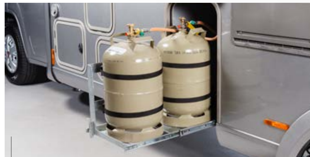
The gas tank box is accessible from outside and positioned at a back-saving height for easy loading. Tanks can be removed separately and are mounted on a pull-out rack, depending on the floor plan.
