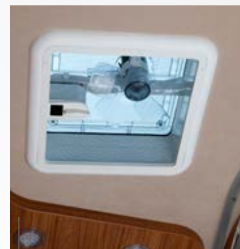
Fiamma Turbo-Vent roof hood with powerful twelve-volt motor.
