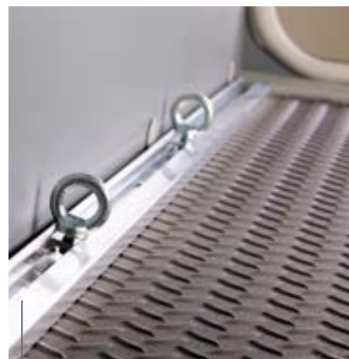
Lashing rail for safe transportation of items in the garage.
