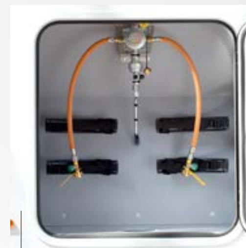
Gas bottle box with optional Duo-Control and Eis-Ex unit.
