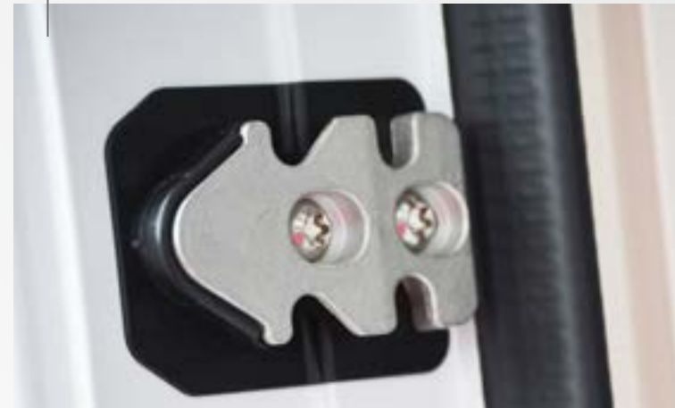
Flush hinges prevent clothing snagging on the vehicle.
