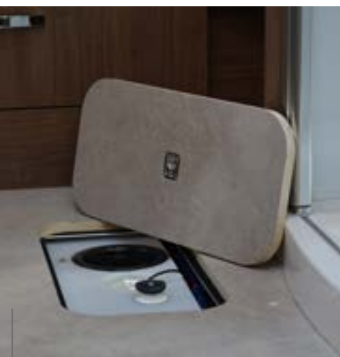
Interior service cover for easy cleaning of fresh-water and waste-water tanks.
