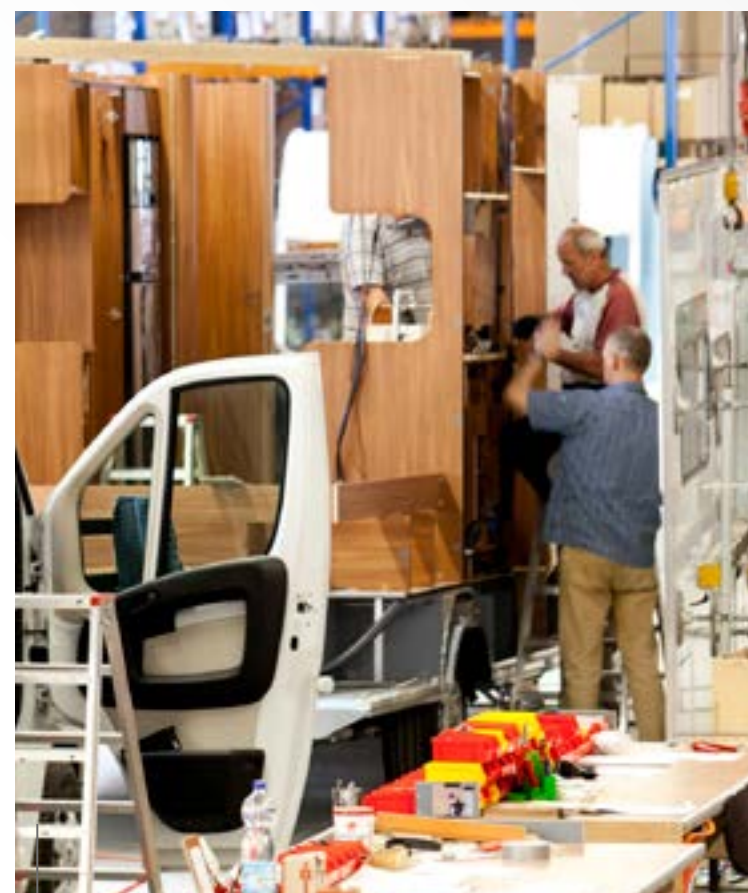
Precision assembly of the separate furniture components.
