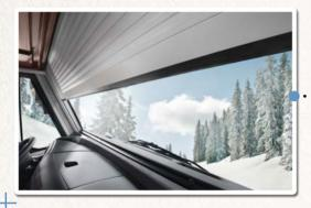
We had to come up with something special for the large panoramic windscreen. They don't come in double glazing. The electrically operated and insulated front blind (optional) ensures that the cold stays outside, even here. The intervening space is also heated directly.
