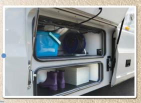
All installations and storage areas in the double floor can be accessed conveniently and in a way that's conducive to service – via the fully insulated bus flaps.
