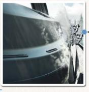
The rear ventilation on the windscreen works in conjunction with the convector heaters like a thermal screen.
