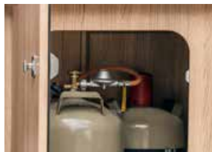
Gas bottle locker for 2 x 11 kg gas bottles (except CLIFF 601 with 2 x 5 kg gas bottles)
