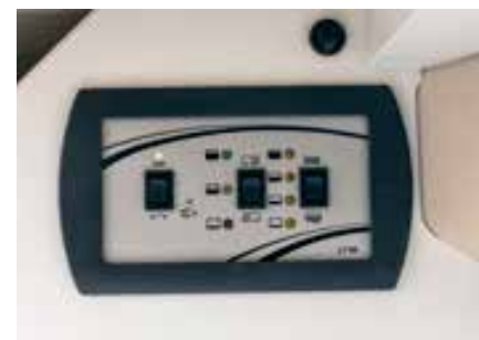
Control panel provides information about water levels and battery capacity
