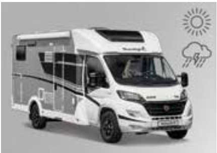
GRP roof and rear panel
