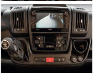
As an integrated on-board system, the new HYMER-SMART-Control connects the main peripheral devices of the Hymer-mobil B-Class SL with the control unit of the navigation system. This enables you to check all relevant data in real time, e.g. the voltage of the starter and living area batteries, the fresh and waste water tank levels and the 230V mains power supply.
