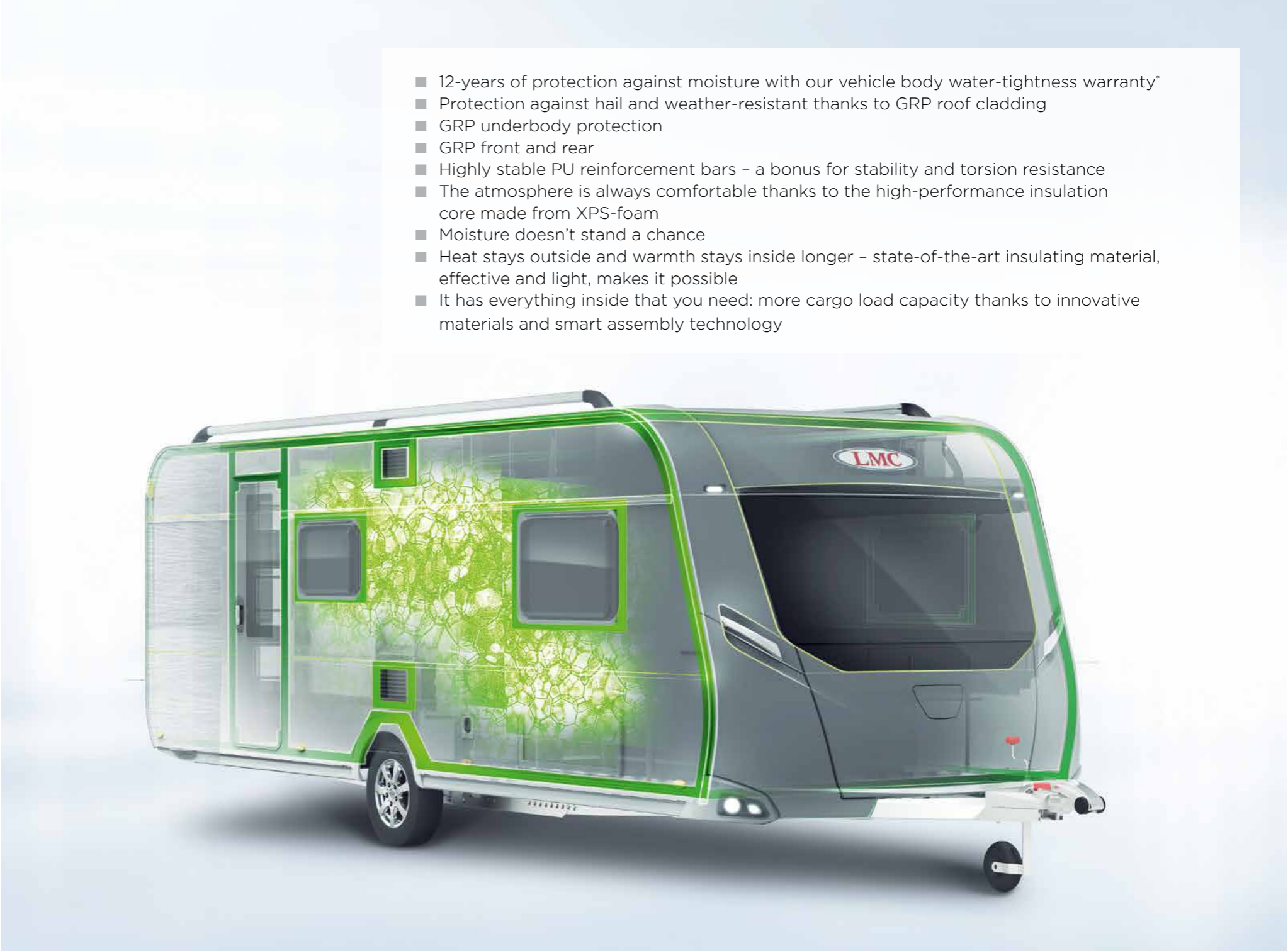
1. Extra-hard PU-core for high level impact resistance
