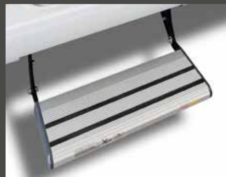
⊕ Cab door with electrically extending and retracting step
