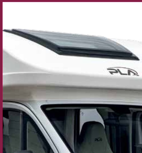
CUPOLINO MONOBLOCCO IN VETRORESINA OVER CABIN IN FIBER GLASS. HUTZE AUS GFK.
