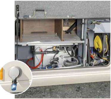
Self-retracting cable reel with 15 m of cable and central supply system
