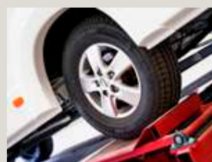
DRIVING DURABILITY TEST Durability tests are performed and simulated with equipment corresponding to 10,000 km of normal driving.
