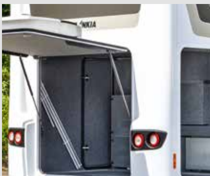
Adjustable rear and side flaps for loading and unloading the storage compartment
