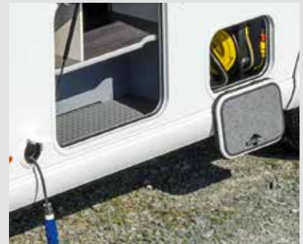
Self-retracting cable reel with 15 m of cable and central supply system
