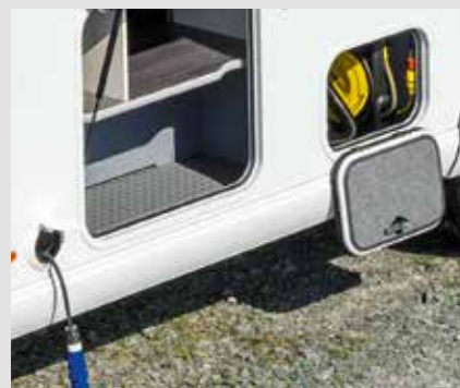
Self-retracting cable reel with 15 m of cable and central supply system
