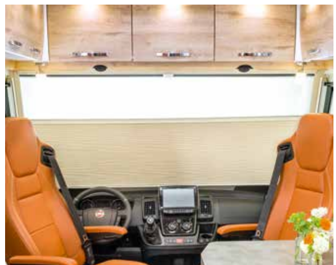
Power front darkening blind with privacy and sun visor function
