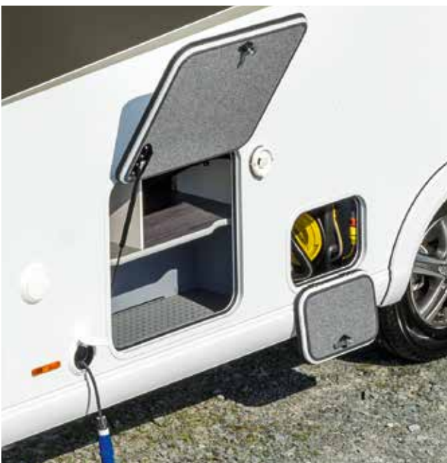
Self-retracting cable reel with 15 m of cable and central supply system
