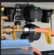
Gas switch-over automatically switches to the reserve bottle when the first one runs out.
