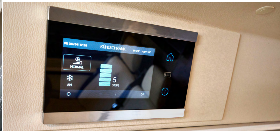
New WESTFALIA electronic control unit with touch-screen for controlling and monitoring all on-board functions.
