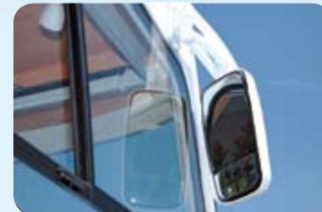
Heated and electrically adjustable outside mirrors (A-Class models)
