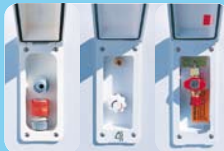
Mains water connection, outside shower and external gas socket
