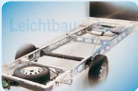
Alko low frame chassis Fiat and Mercedes (6400/6800/7900 6t/8400 6 t)
