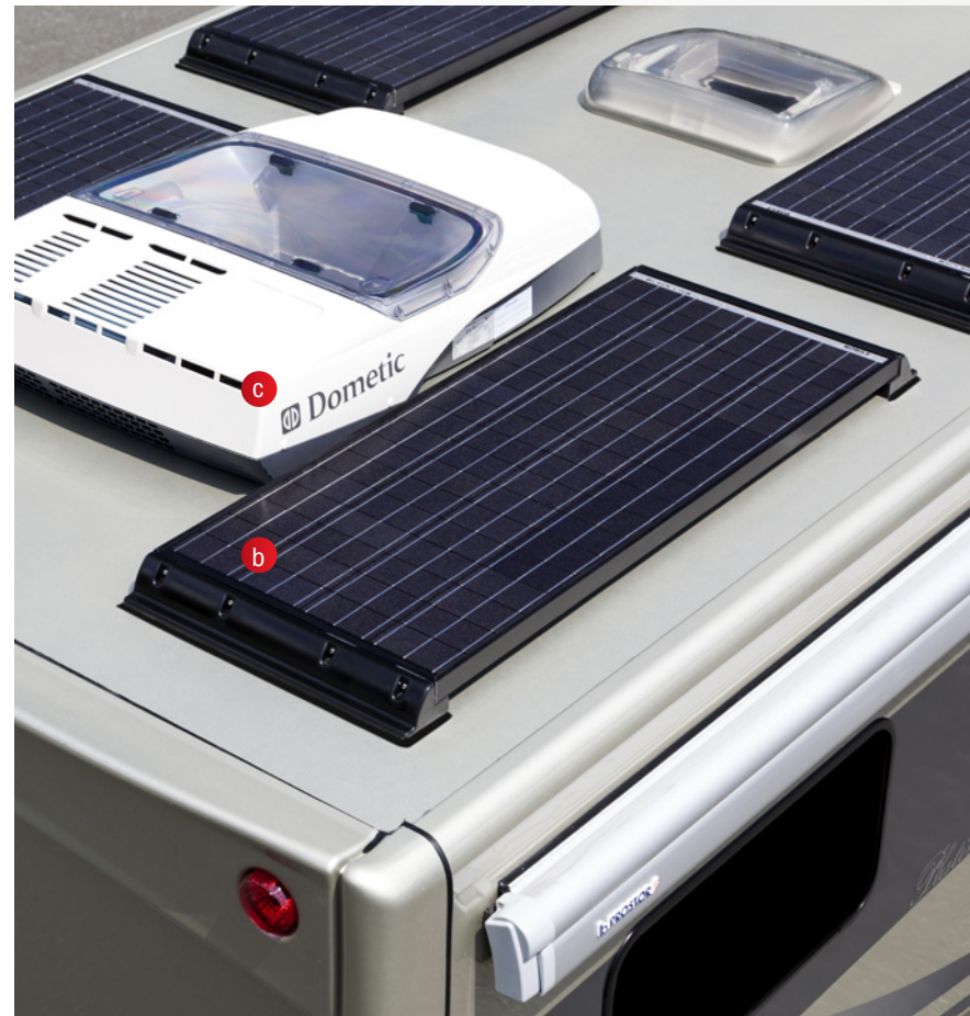
a BÜTTNER ELECTRONIK - comprehensive technology package b 72-cell solar module c Dometic Freshlight (option) - roof air conditioning and skylights in one
