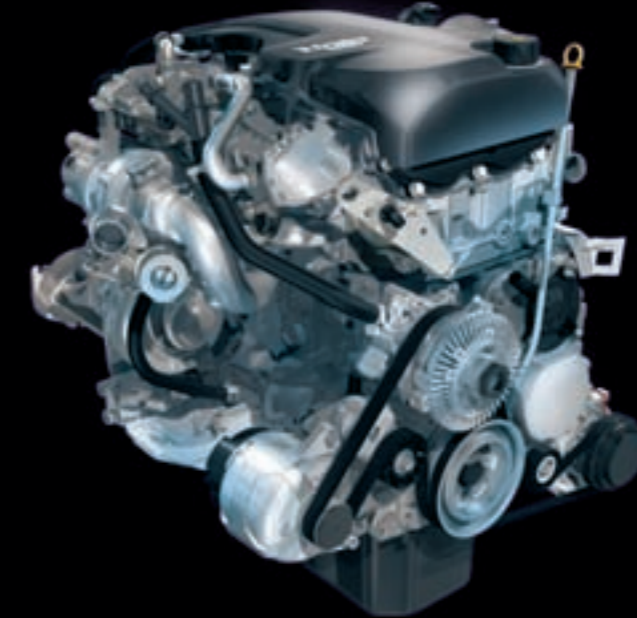
3.0 litri Common Rail - Twin Turbo
