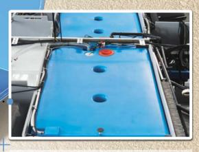
The large water tanks are mounted in the heated double floor insulated with a double-sided aluminium sandwich and so won't freeze at sub-zero temperatures. The water tanks can be removed and replaced via the rear garage.
