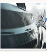
The rear ventilation on the windscreen works in conjunction with the convector heaters like a thermal screen. The optional Seitz S7 windows are double-glazed. They are easy to operate with one hand and have thermally broken aluminium outer frames.
