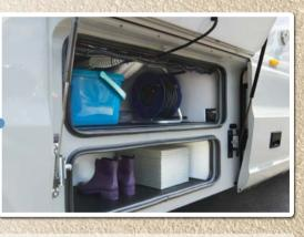
All installations and storage areas in the double floor can be accessed conveniently and in a way that's conducive to service – via the fully insulated bus flaps.
