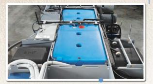
Optimum axle load is a given as the weight of the installations is distributed across the double floor just so; the two large water tanks, for example, are located in the centre of the rear axle.
