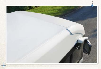
The flush-mounted transition from the front mask to the roof prevents backpressure of water and ensures that the water runs off to the front.
