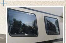
The optional double-glazed side windows ensure better insulation and also offer up to 80% more heat protection than conventional, single-glazed side windows.
