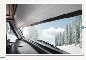
We had to come up with something special for the large panoramic windscreen. They don't come in double glazing. The electrically operated and insulated front blind (optional) ensures that the cold stays outside, even here. The intervening space is also heated directly.
