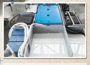
The underfloor is made entirely of double-sided aluminium sandwich. The upper floor serves as a heatstore and ensures that the interior of the vehicle is very well insulated.
