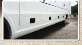
The elaborate side skirts made of varnished aluminium profiles give the Flair a sporty look on the outside. They cover the chassis frame and the retracted outside step.
