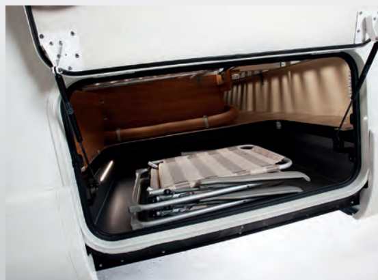
<< New: Gas strut supports for exterior access doors for ease of operation
