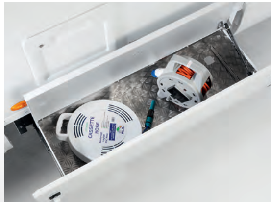
<< New: Pull-out underfloor drawer for a water hose and electric cable reels
