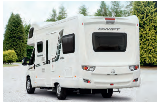
⤴ Closed-mould GRP rear panel for smooth finish, strength and ease of repair
