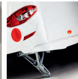
Heavy duty rear corner steadies and profiled skirts
