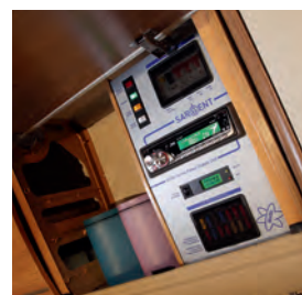
<<Locker mounted eye level power supply unit and power management for easy access
