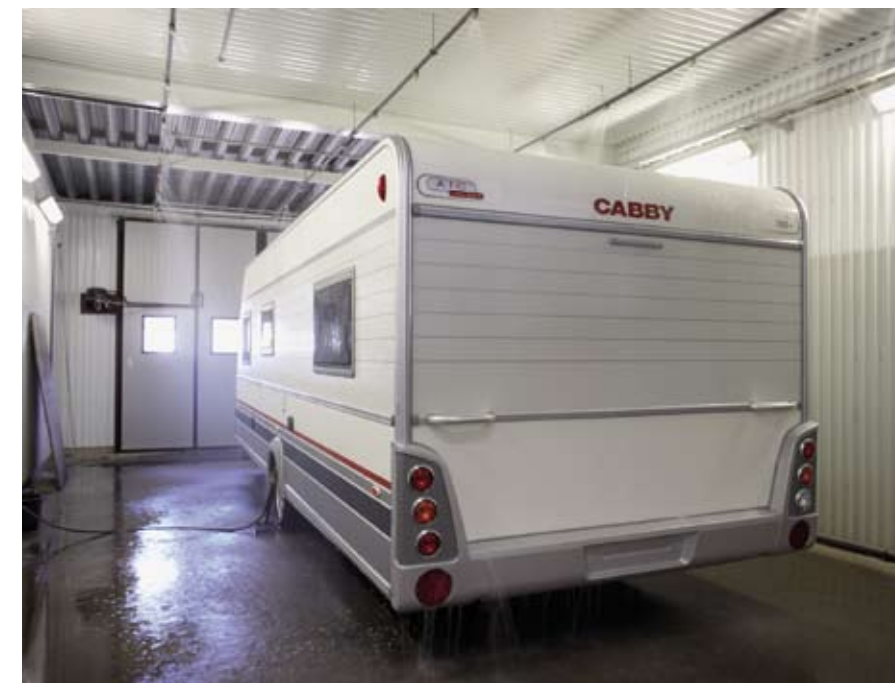
OK – we admit it. The sun doesn't shine every day in Sweden. That's why we give all our caravans a water test before they leave the factory. Then we know that everything is in perfect working order and that as a customer you can feel safe and dry during all your years as a Cabby owner.
