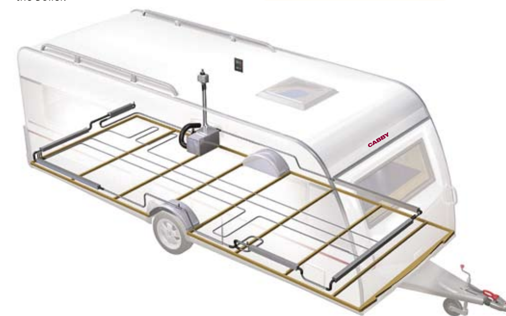
The coils in the underfloor heating are particularly effective as the heating plates in the floor distribute the heat evenly.
