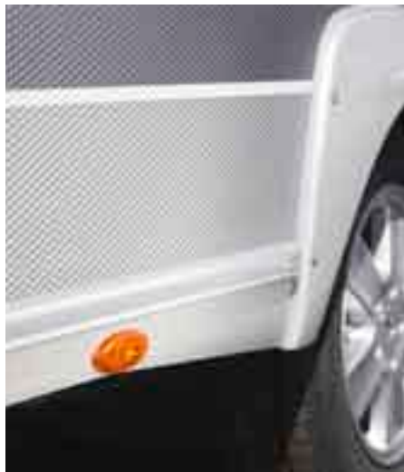
Above: Aluminium skirts with integrated side marker lights.
