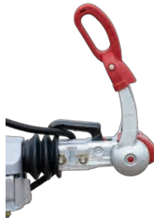
The AKS stabiliser hitch provides a stabilising effect by means of a friction lining that presses against the car's tow ball.
