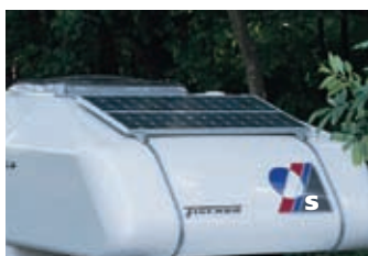
Solar system consisting of a 75-W module, charge current controller
