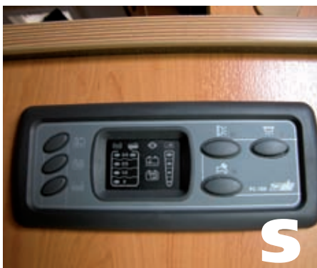
On-board control system for fresh/waste water tank, Box/vehicle battery, 12 V main switch and water pump switch (not on TRAIL / BOX 200)
